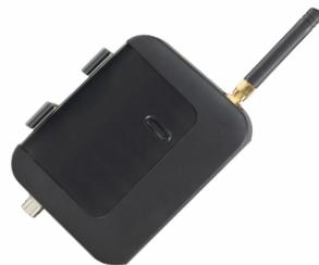
Designed to provide connectivity to X-Consoles (X25 and X35), the CL-10 cloud connectivity device offers Topcon technology owners a simple, integrated and cost-effective path into digital farm management.
